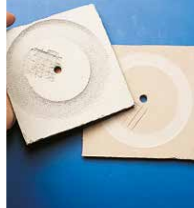
Taber abrasion executed on Ultraplan (right specimen) and on conventional levelling (left specimen) after 200 cycles
